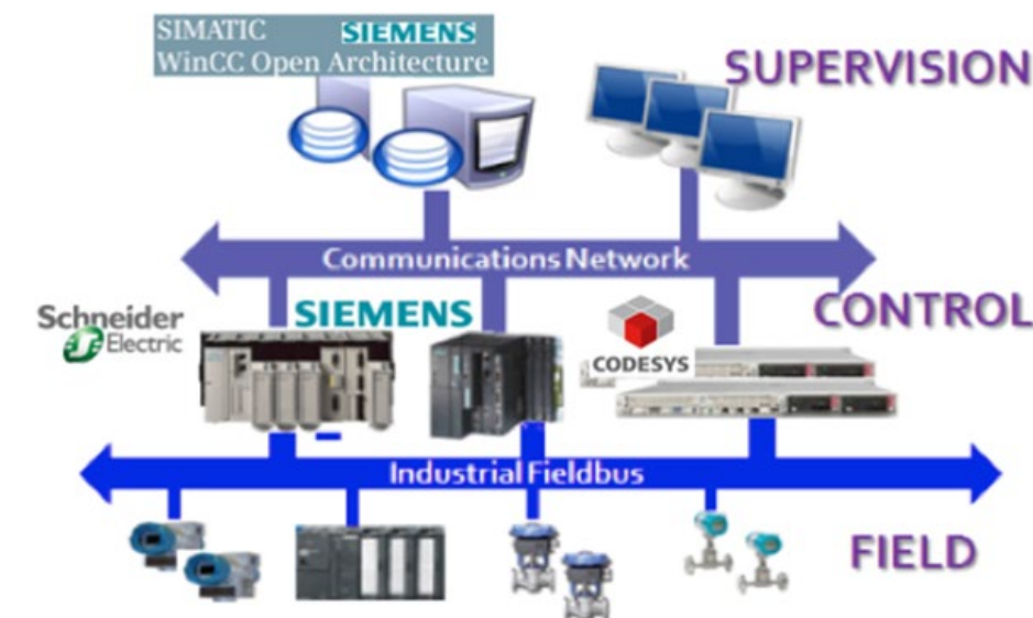
Figure 44: Typical industrial control layer configuration
