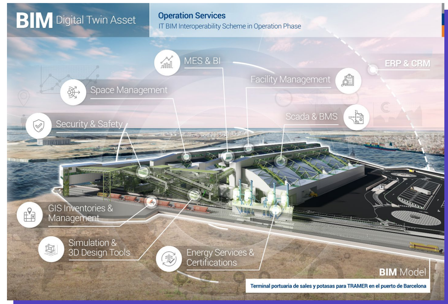
Figure 1: Conceptualisation of a Building Digital Twin Instance Interoperability Services (sketch by: M.Borràs)
