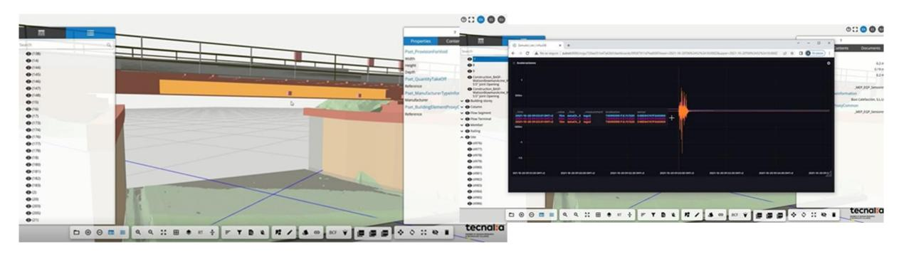
Railway Bridge monitoring through the integration of IoT sensors, IFC model and structural analysis algorithms.
